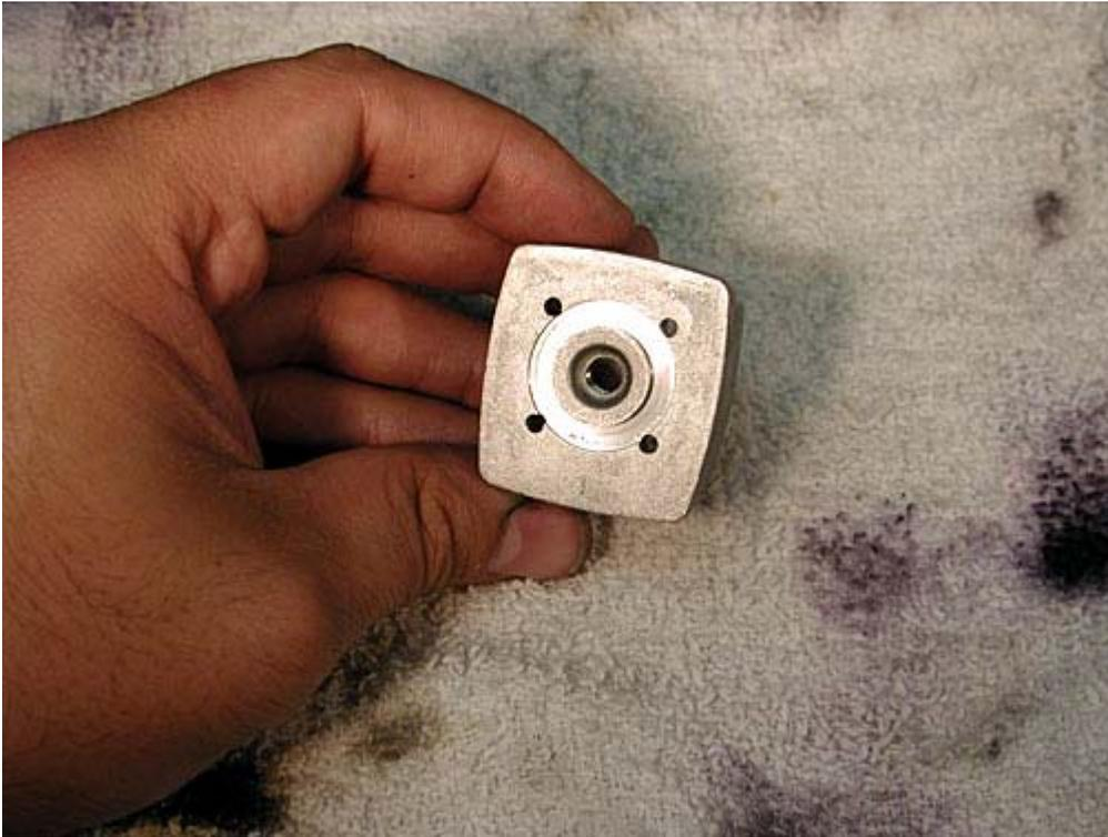
Get the new head shim and gently lay it in place. If it was slightly bent in transit, it's okay, the pressure from the head will hold it flat in place.
