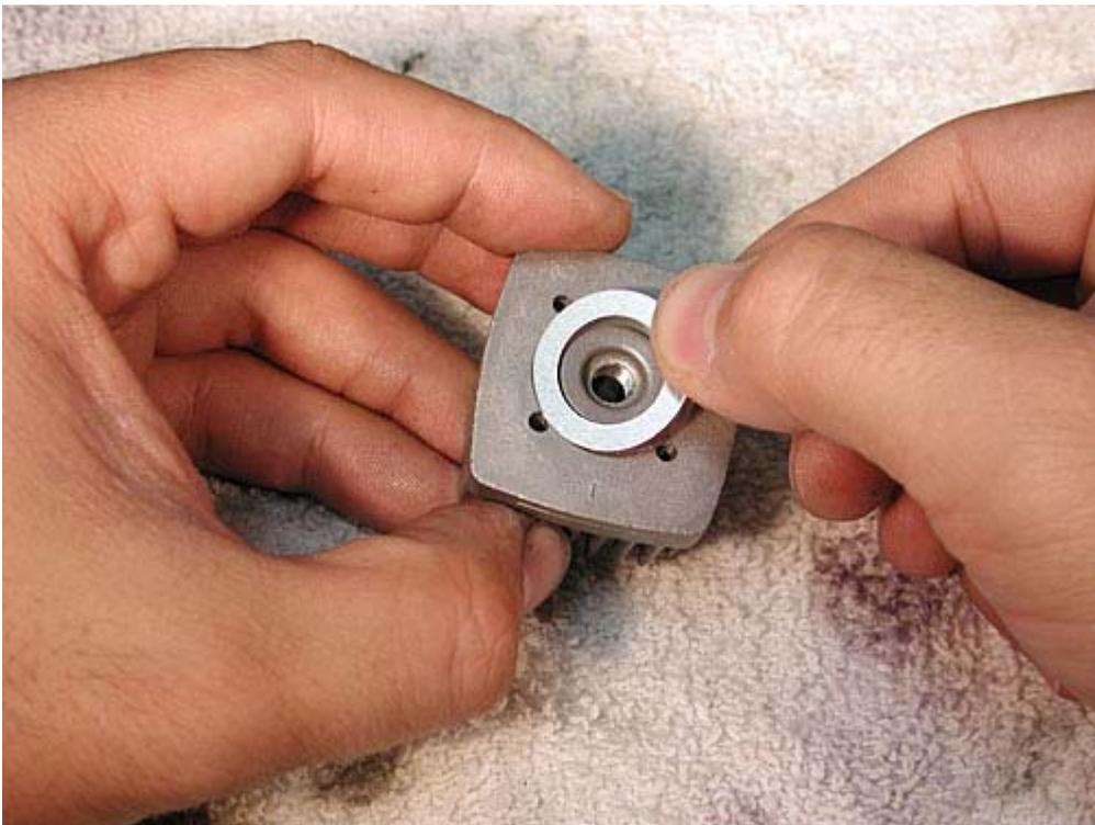
Carefully install the head as shown below, so the head shim doesn't fall off the head.
