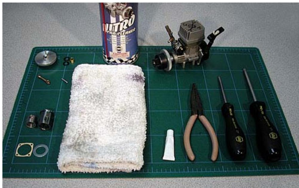
Hardened-tip screwdrivers are highly recommended, they lessen the chance of damaging the screw heads and the screwdriver tips and last much longer than "bargain bin" screwdrivers.
