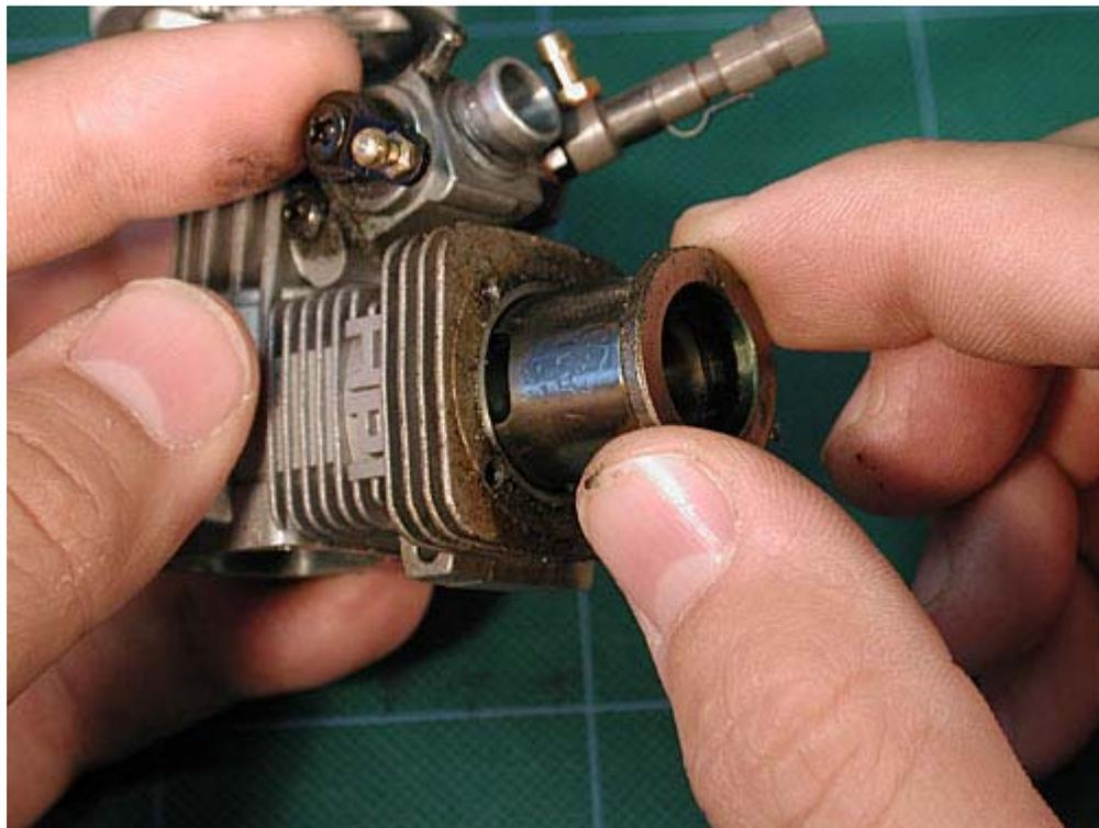
Move the flywheel back and forth until the cam is at the bottom of the engine case, as shown.
