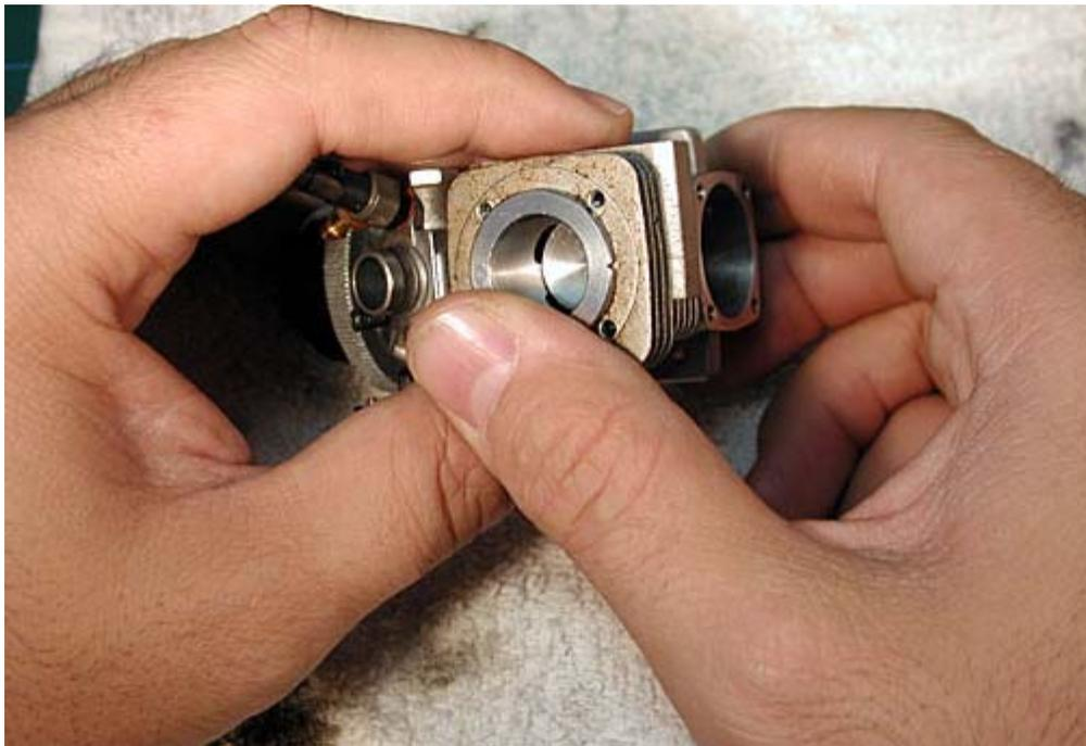
Set the engine case aside. Get the engine head and pull out the head shim with a hobby knife.
