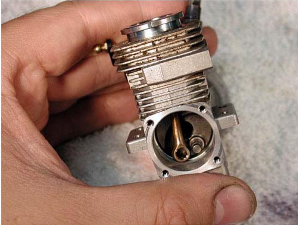
Push the sleeve only partially into the engine case as shown below.
