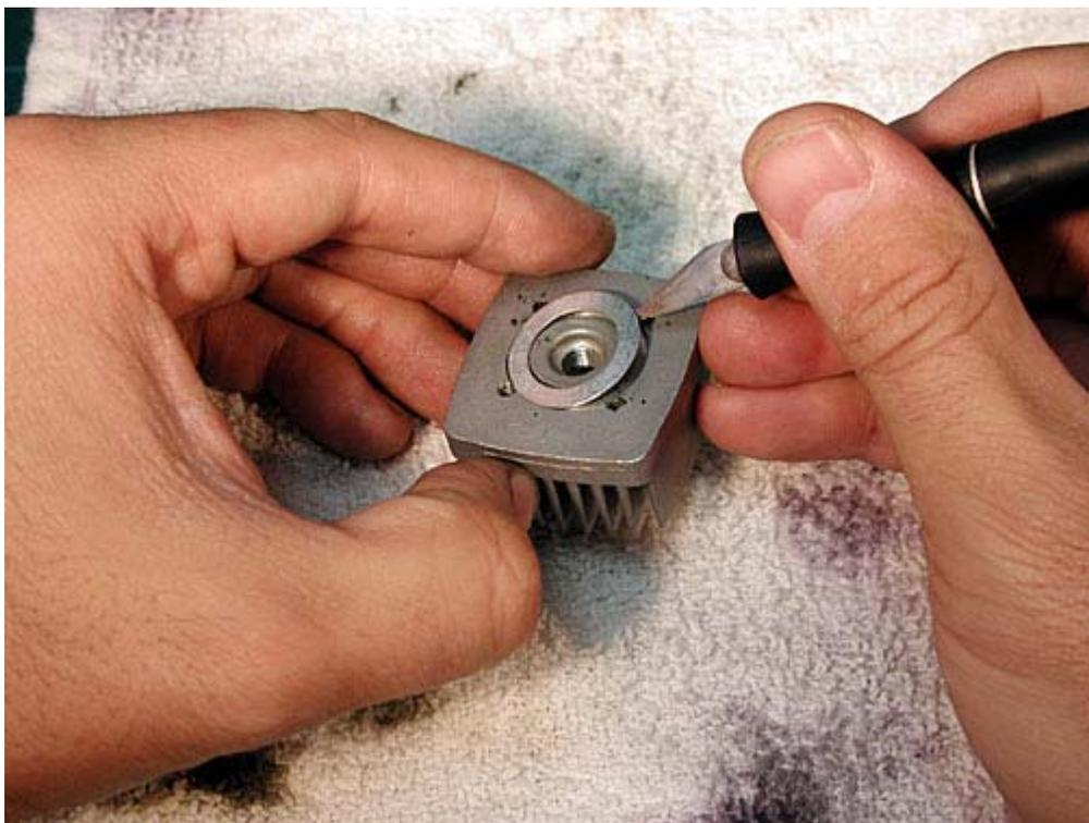
Use Nitro Car Cleaner to spray away any dirt from the screw holes and bottom of the head.
