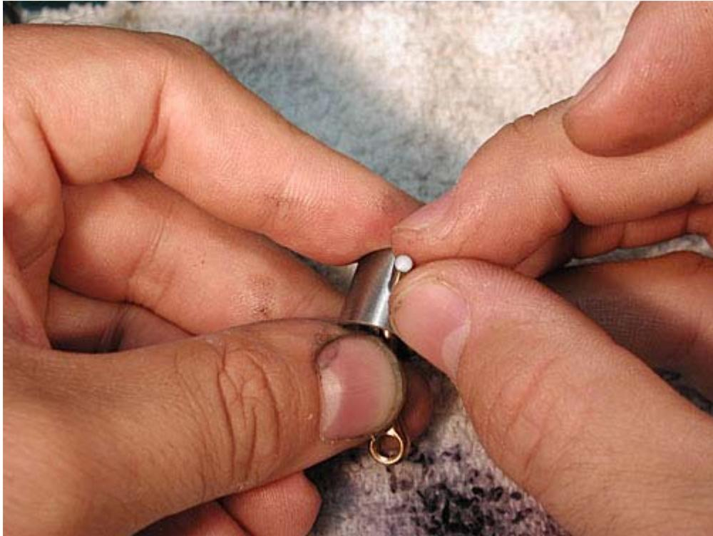
Notice that the 15FE wrist pin has white plastic on one end and is plain on the other end. The white plastic is Teflon; this end of the wrist pin should face to the outside of the piston. Now slide the wrist pin through the piston hole and through the con rod. Make sure the white end faces to the outside, as shown. If the engine you have uses wrist pin clips, make sure to attach those now.
