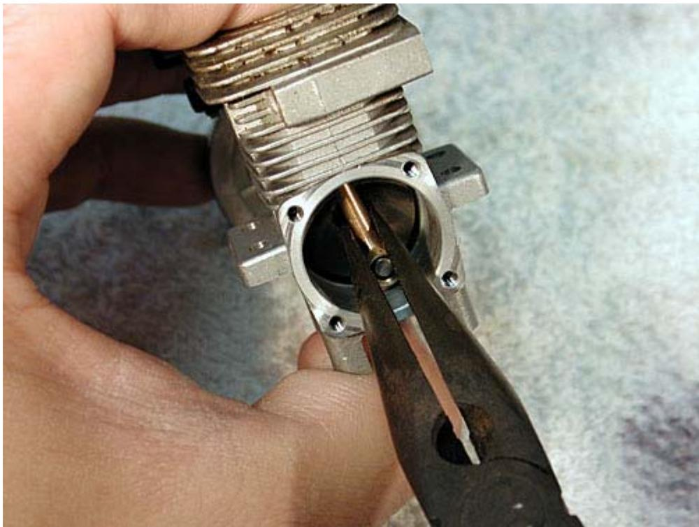
If the piston comes out of the bottom of the sleeve while you're positioning the con rod, don't worry. Use a hobby knife to gently push the piston into the sleeve again.
