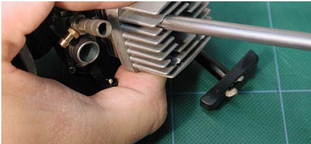
Now that you have the heat sink head off, set it aside also. Remember the way the fins faced so later on you won't have to reposition the head after you install it in your car or truck.
