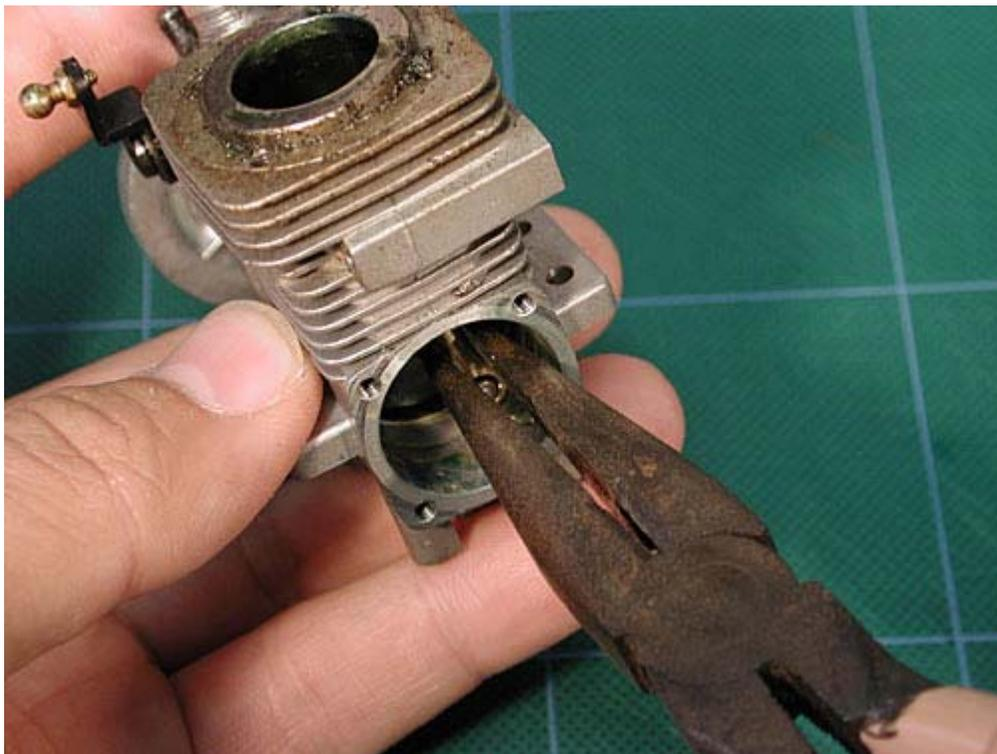
Pull the piston and connecting rod out from the top of the engine case.
