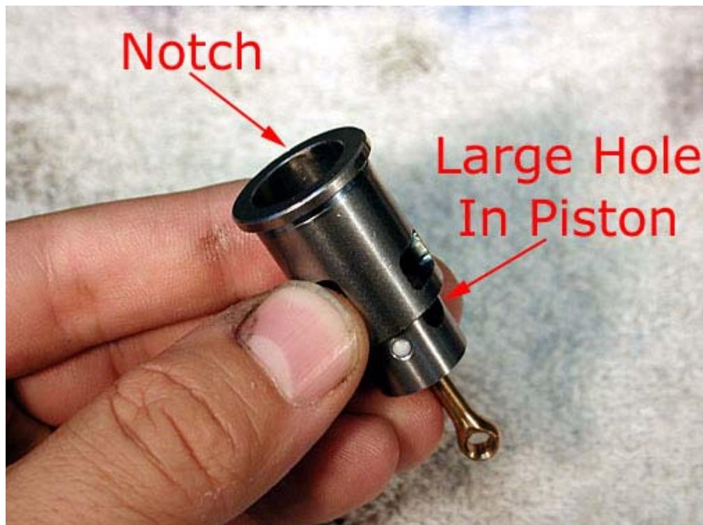
Carefully insert the sleeve (with piston installed) partially into the engine case. Make sure the notch in the sleeve faces the rear of the engine case. Remember, the "front" of the engine is always the side with the flywheel, clutch, etc., and the "rear" of the engine is where the pullstarter or backplate sit.
