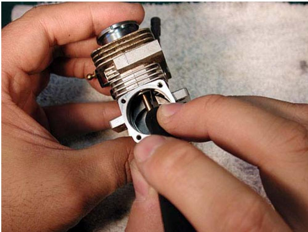
Push the sleeve all the way down into the case. Make sure the notch lines up with the seam of the case, again, facing to the rear of the engine.
