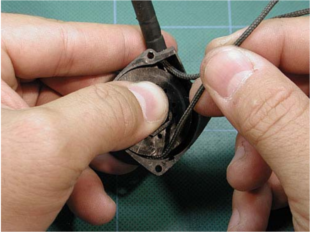
Pull the entire length of cord out from the inside of the pullstarter housing.
