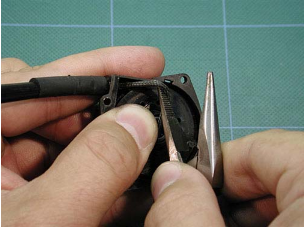
Continue to hold firmly on the spring assembly as you pull out all of the cord.
