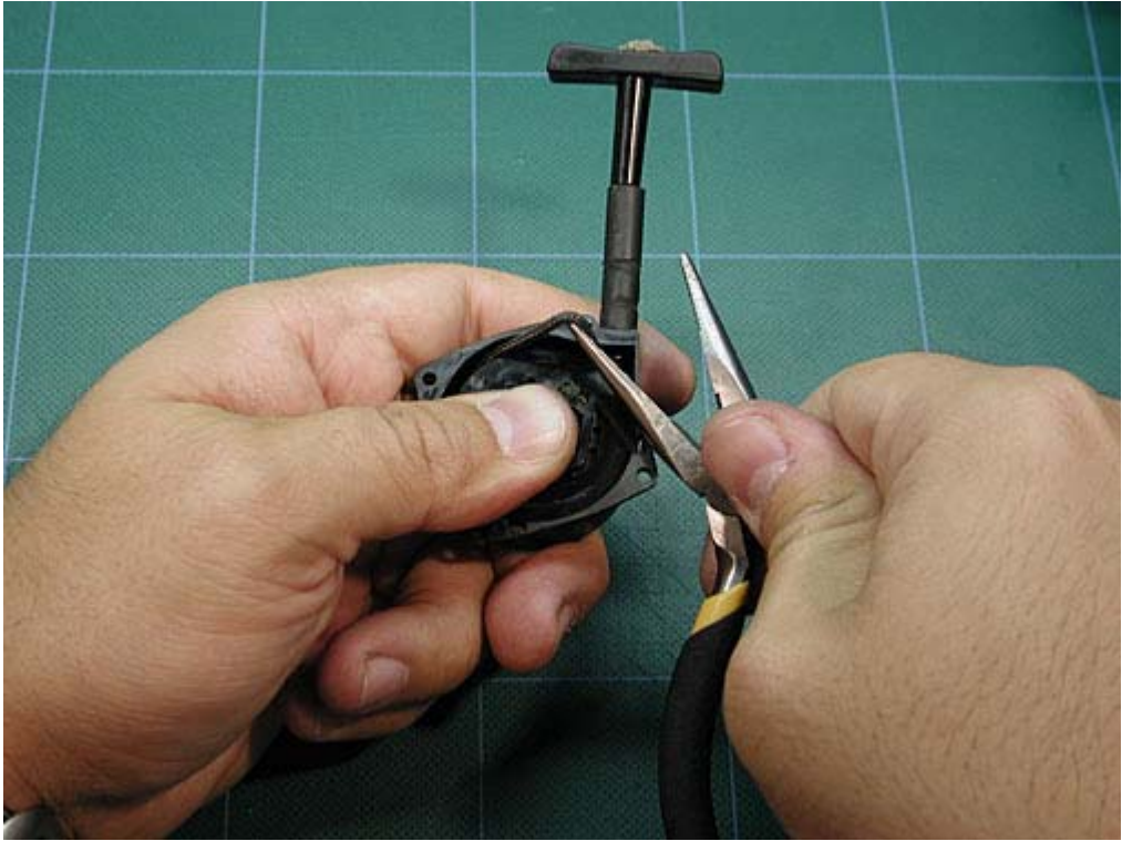
Untangle the cord again and take the twists out, then slowly let the cord retract.
