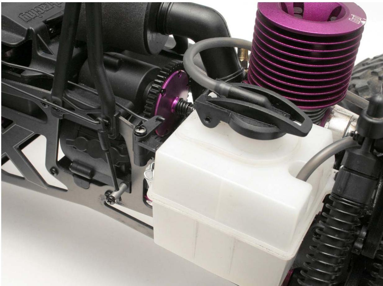
Replace the fuel tank, fuel lines and the R clips and you are good to go!
