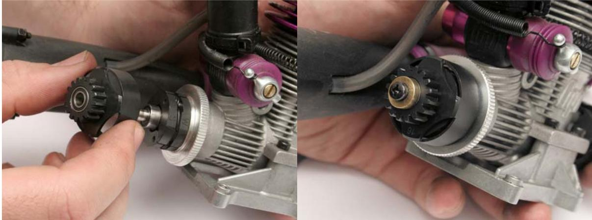
Fit the Racing Clutch Bell, remember to use thread lock on the screw
