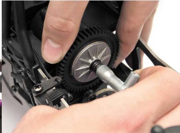
Undo the nut that holds on the slipper clutch
