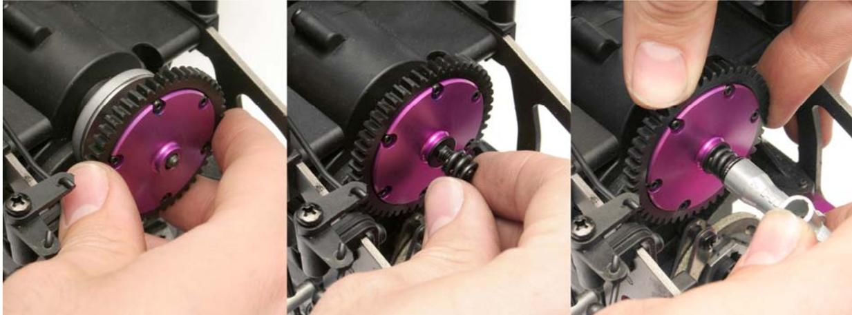
Fit the new spur gear and replace the washer, spring and nut
