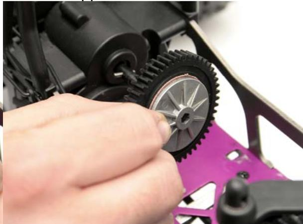
Remove the spring, washer and the slipper clutch parts
